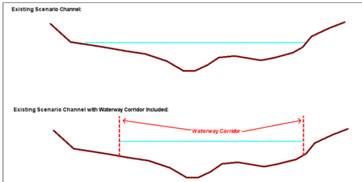
Figure 6-1: Implementation of Waterway Corridor using 'Walling Off' Method
